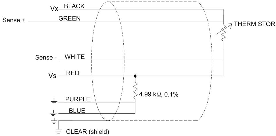
FIGURE 7-3. 110PV schematic
