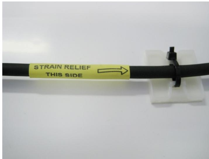
*FIGURE 7-1. 110PV strain relief label*
